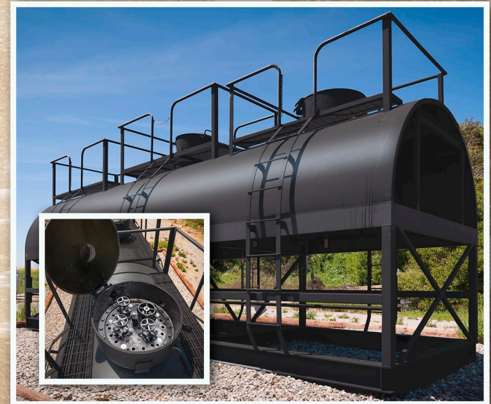
3 DOME RAIL CAR TRAINING SIMULATOR WITH CHLORINE, PRESSURE, & GENERAL SERVICE DOMES
